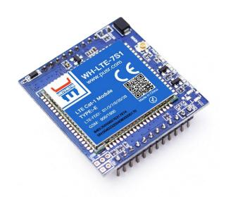
WH-LTE-7S1 is a LTE Cat 1 communication LTE module, which supports and GSM. WH-LTE-7S1-E covers the mainstream frequency bands of European operators. It has perfect software function, supports TCP/UDP transparent transmission, SMS transmission and configuration, and also supports HTTPD Client mode and AT command configuration. At the same time, it supports MQTT(S).
