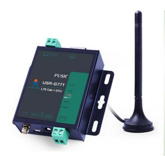
USR-G771 is an LTE CAT 1 cellular modem, which supports LTE and GSM. USR-G771-E covers the mainstream frequency bands of European operators. It has perfect software function, supports TCP/UDP transparent transmission, SMS transmission, TLS/SSL encryption transmission, HTTPD Client mode, and AT command configuration. Also, it is simple to configure, has high reliability and built-in hardware watchdog, supports FOTA upgrading.
