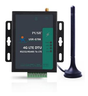
USR-G786 is an LTE Cat 4 Modem with low latency, high reliability and high real-time characteristics. The product has a fast transmission rate, with an uplink peak rate of 50Mbps and a downlink peak rate of 150Mbps. USR-G786-G supports the frequency bands of major operators all over the world, USR-G786-EUX in European, and USR-G786-AUX in Australia and Latin America.
