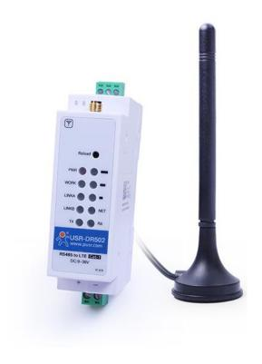
USR-DR502 is a LTE Cat 1 communication modem, which supports LTE and USR-DR502-E covers the mainstream frequency bands of European operators. It has perfect TCP/UDP software function, supports transparent transmission, TLS/SSL encryption transmission, SMS transmission, HTTPD Client mode and AT command configuration. In addition, it is simple to configure has high reliability and built-in hardware watchdog, supports FOTA upgrading.
